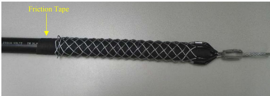
Picture 1: Friction Tape Applied Between Grip and Cable
